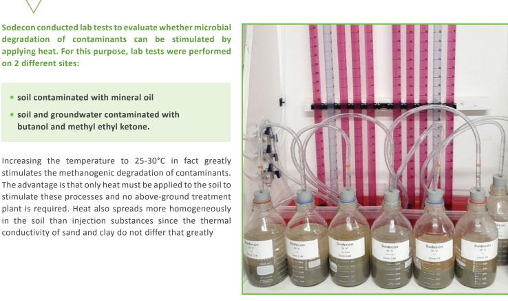
Lab tests were performed in which the volume of biogas formed by the degradation of the contaminant was collected. By monitoring this volume, an estimate of the biodegradation could be made. It was found that the decomposition of mineral oil could be accelerated by a factor of 3 and that the decomposition of butanol and methyl ethyl ketone could be accelerated by a factor of 2 to 5 by applying heat.
